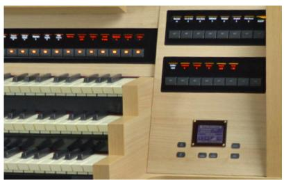
disposition of the organ running Under the Hauptwerk computer program. The system display is conveniently located on the right side of the instrument with its own set of easy to use controls. There are plenty of pistons (expandable under request) available for both divisional and general memories which are carefully positioned on the instrument to allow a wide range of possibilities and personalization, all at your fingertips.
