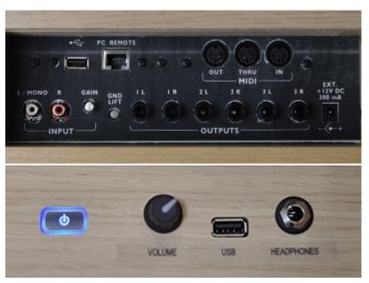
Master volume, headphone jack, USB host pen drive for saving-uploading settings, and MIDI song recording and playback, are all conveniently located on the front of the organ.
